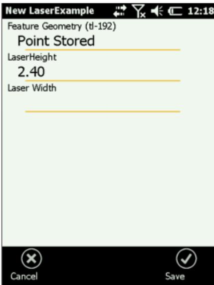
To fill in the Laser Width field press the Laser Rangefinder button again. This time change the Workflow to *2 Shot Width*. Start from the Left to Right of the object.
